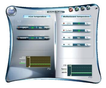
On the underside, it shows the graphs of the temperatures. Only the curves of the item which the button is lit up with red color will be shown.
